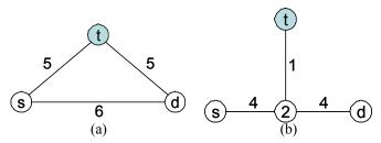
Fig. 2. Example networks with request (s, d, 5). (a) There is a feasible path through regeneration node t. (b) There is no feasible simple path.
