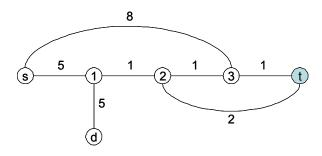
Fig. 5. An example wherein the concept of non-dominance fails for impairment-aware routing. The request is (s,d,9) and node t is a regenerator.
